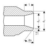
Butt-weld ends to DIN 3239 2-R3, edge form to DIN 2559, code no. 22
